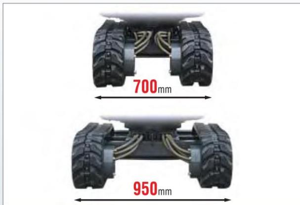
With the widest ranging spanners in its class, the machine can access into tight spaces to ensure a very high level of work performance.
