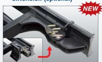
The blade width can be easily adjusted, offering you the flexibility to fit the job. Adjustment is simple and easy with the two fastening pins.
