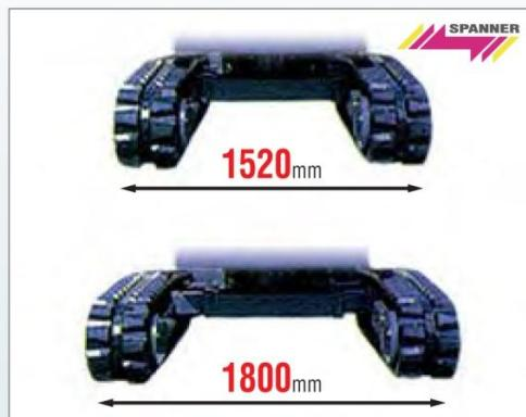
Due to the unique design, the crawler width ranges from 1520mm to 1800mm, which enables to transport easily and to fit into tight work sites. This also provides outstanding balance and stability yet in wider work sites.
